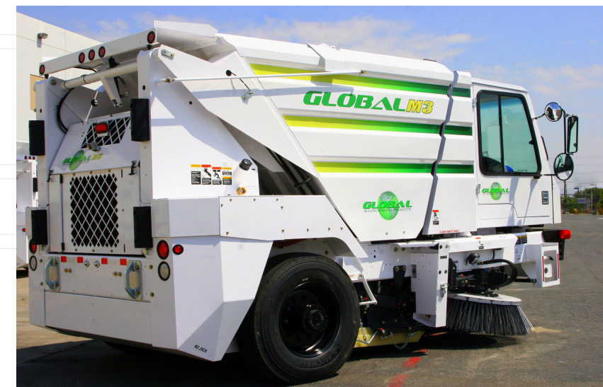
ABOVE The Global M3 is designed to make routine maintenance easy, so your sweeper spends more time on the street and less time in the garage. Two swing-out center body panels provide unrestricted access for elevator adjustment, maintenance and daily cleaning.
