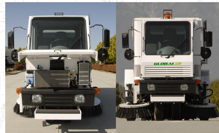
RIGHT The Global M3 features many maintenance-friendly attributes, such as a rear swing-out radiator, easy access front mounted AC condenser, brake and windshield washer fluid reservoirs, and cab fresh air filter.
